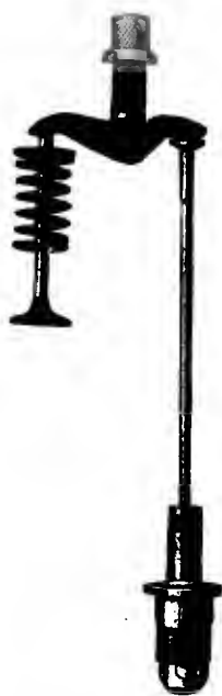
Assembling of valve reciprocating parts. Note adjusting screw and spherical fulcrum at top, roller valve-lifter at bottom.
